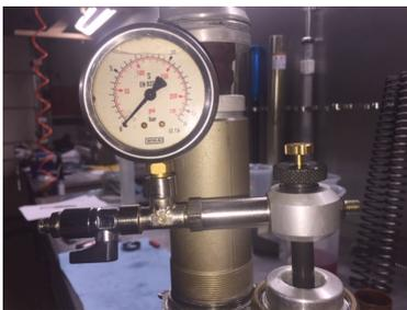
1) AVVITARE IL PRESSURIZZATORE NELLA VALVOLA SCHRADER E APPOGGIARE APPENA UN PO' LA GOMMA DI TENUTA INTERNA.
