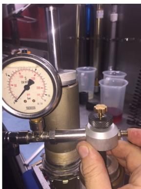
6) UNA VOLTA RAGGIUNTA LA PRESSIONE VOLUTA, SVITARE IL POMELLO ORO E PORTARE LA PRESSIONE A ZERO NEL MANOMETRO TRAMITE LA VALVOLA LATERALE.
